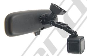
4 - Install the GoPro onto the mount. After all adjustments are made, be sure to check that the hinge pivot adjustment screws are tight. Grab the long arm of the allen wrench to assure that these screws are securely tightened. NOTE: The mirror stem may move side to side while adjusting, make sure the stem pionts straight ahead so the camera does too.
